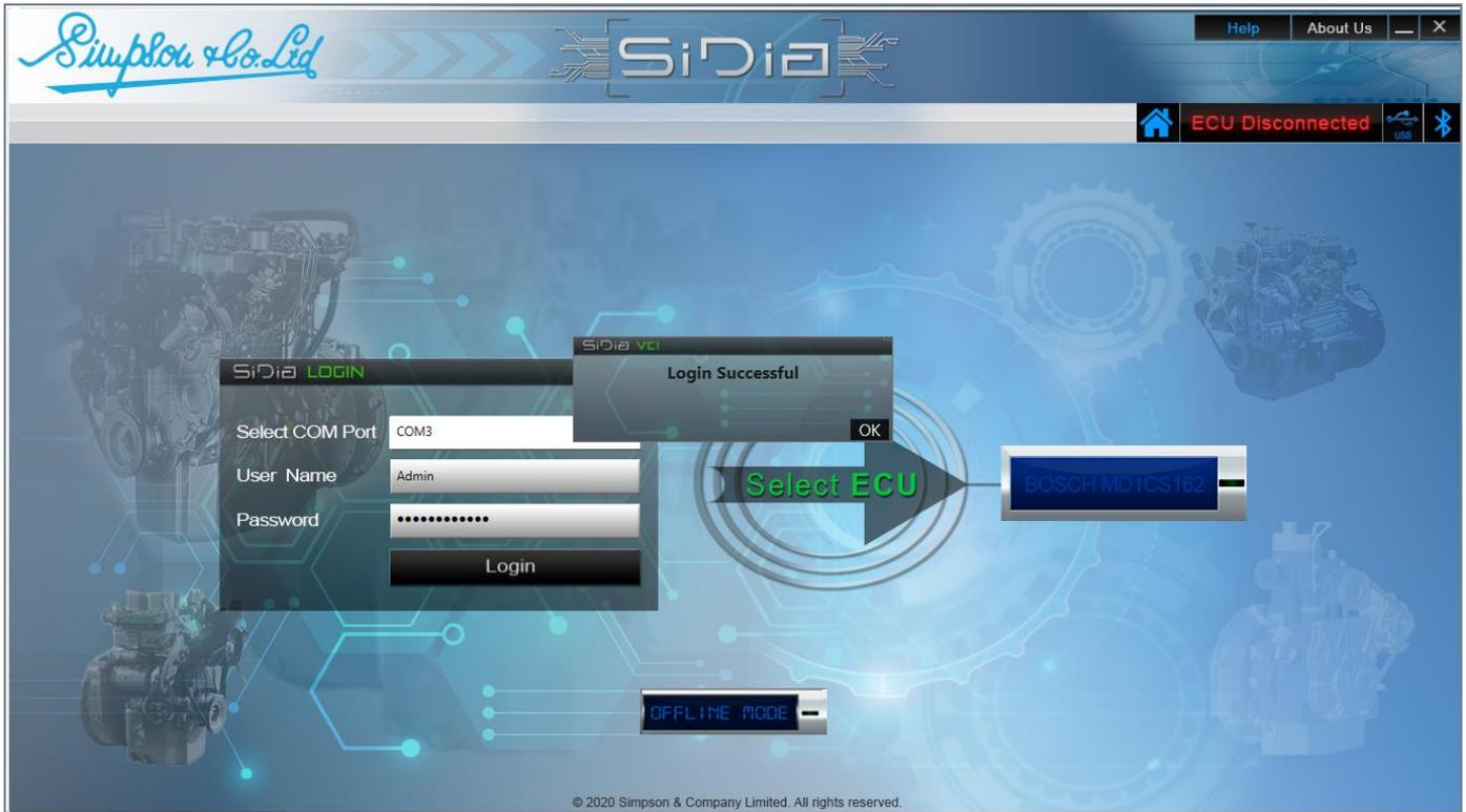
**Step 5:** Select the ECU Type- Bosch MD1CS162 to start the communication with the ECU. If the Communication is established then ECU Details page is loaded. If the ECU is Not Connected/Ignition is Off then ‘Failed ECU Communication...! Please Turn ON Ignition and Try Again.’
