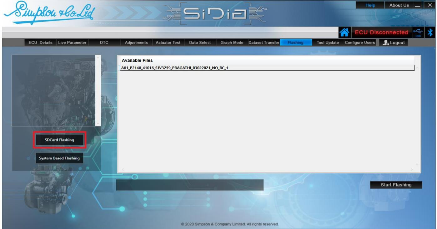
**Step 24:** Click on Start Flashing. Flashing Process is being displayed in the Flashing Status window.
