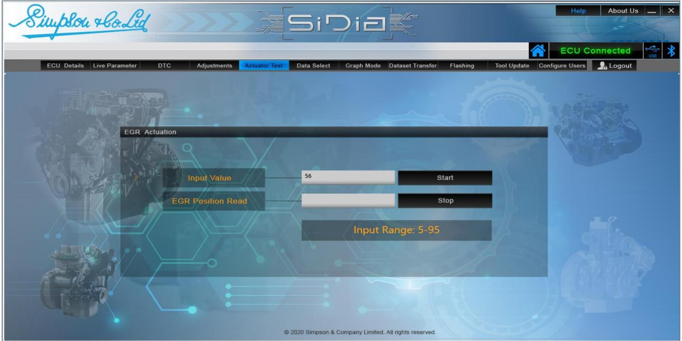
If the Actuator is started successfully then 'Test Activated' pop up message is displayed and if the Test Preconditions are not met or receive any Negative Response from ECU then respective Negative Response pop up message is displayed.
