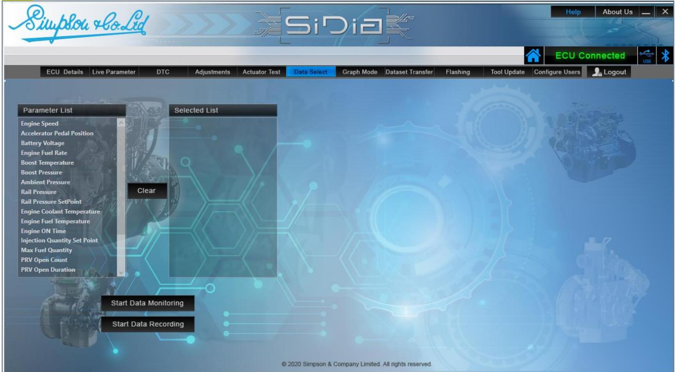
To select the parameters double click on the parameter. The Selected parameter list is displayed in the Selected List box as shown in the image below.
