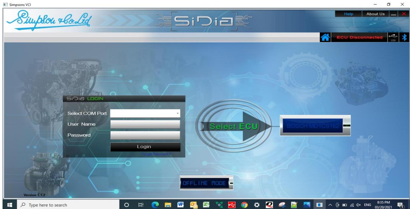
**Step 3:** Offline Mode to be used only if the User need to update the firmware or transfer the dataset without connecting to the ECU.
