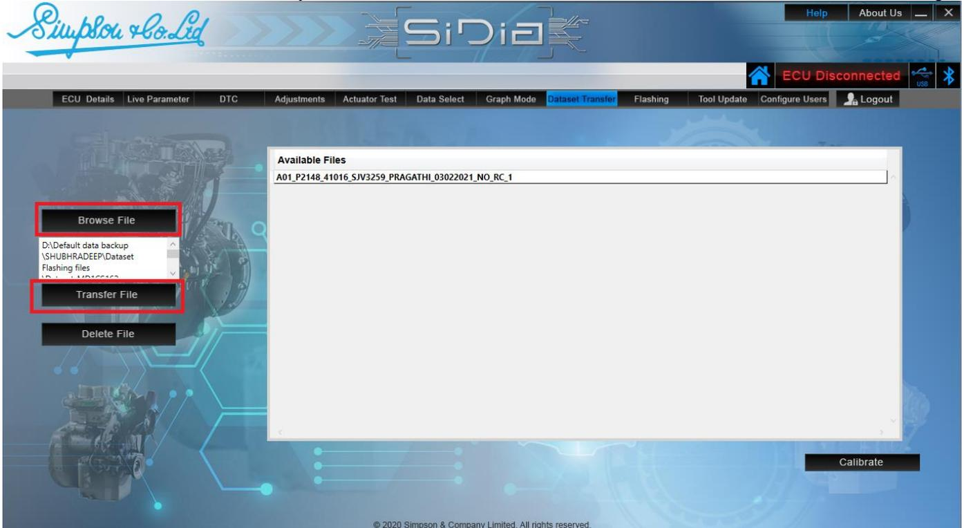
The application is logged out automatically while the Dataset Transfer operation is performed. On Completion of Dataset Transfer the 'File Transfer Completed' message pop up is displayed.
